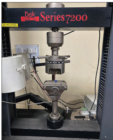
Figure 2: DAK System Inc Series 7200 Universal testing machine
