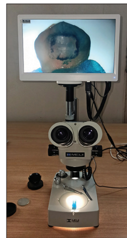
Figure 3: Assessment of the ARI using a stereomicroscope
