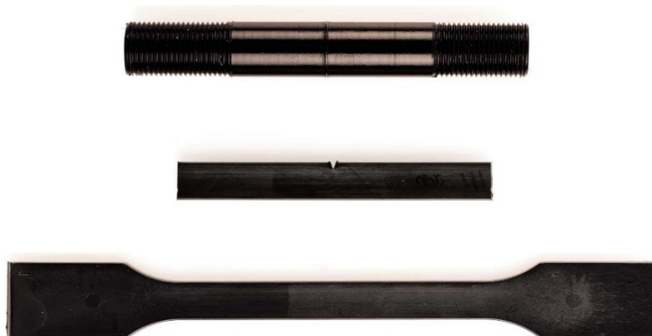
Figure 2. Image of the specimens used in this work made from B75 from top down: CRB specimen lathed from a pressed plate, Type 1 Charpy specimen cut from an MPS, and injection-molded MPS.
