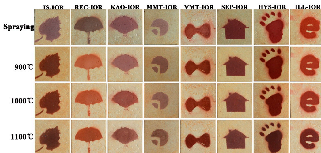
Figure 9. Digital photos of sprayed coatings on ceramic substrate after calcinations at different temperatures (900 °C, 1000 °C, and 1100 °C).
