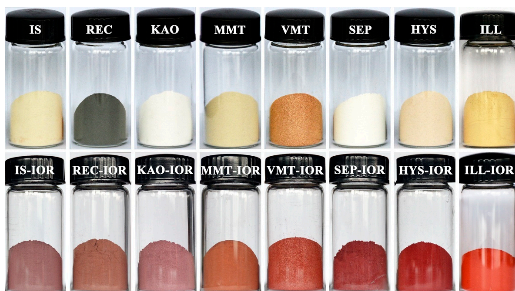
Figure 6. Digital photos of the used natural clay minerals and the corresponding hybrid pigments (For interpretation of the references to color in this figure legend, the reader is referred to the web version of this article).
