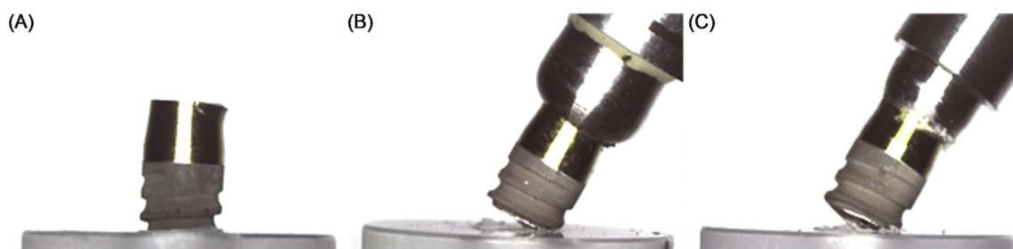
**Figure 4** Failure modes in a static load test: (A) AL: Abutment Level without ferrulized neck; (B) IL<sub>s</sub>: Implant Level with ferrulized neck and screw-retained crown; (C) IL<sub>c</sub>: Implant Level with ferrulized neck and cement-retained crown.
