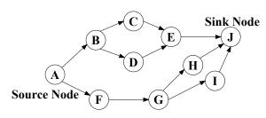
Figure 8. Partially disjoint paths established by MCMP.
