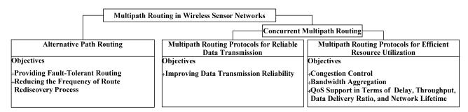
Figure 2. Taxonomy of the existing multipath routing protocols in wireless sensor networks.
