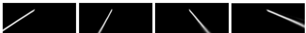
Figure 6. Predicted lane line probability pictures. We can see that different lane lines are predicted for different feature map channels, and some key points are selected and reconnected to obtain the final prediction map.
