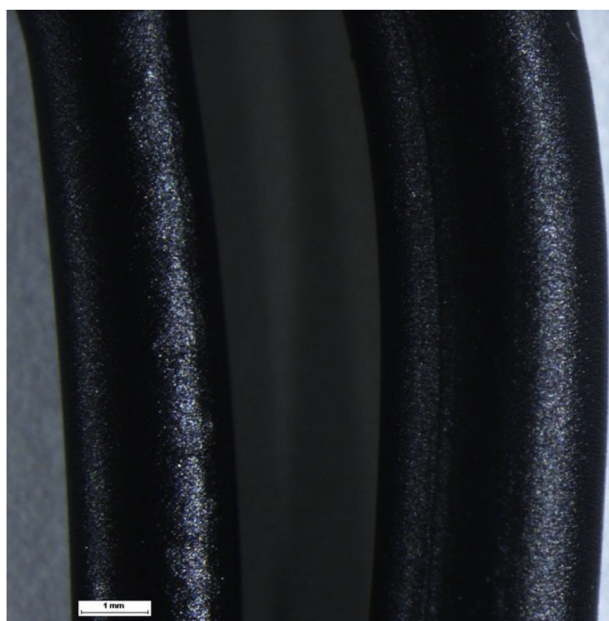
Figure 8. General photograph of the post extrudate: left composite with 15 wt.% talc at 190 °C/5 kg load and right HDPE base material at 220 °C/12.16 kg load.
