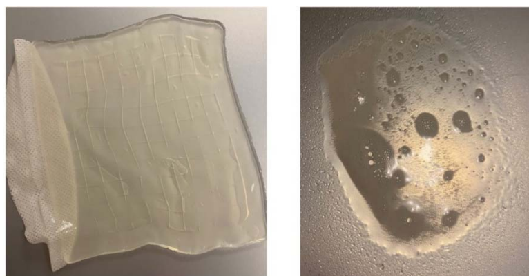
Figure 6. Types of hydrogels. On the left , an inert hydrogel in a sheet. On the right a semi-liquid, amorphous form.
