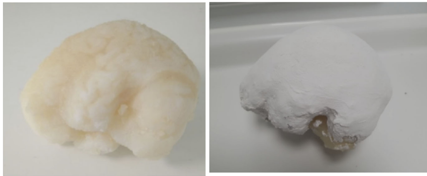
FIG. 1. Three-dimensional printing brain (left) and the completed phantom after coating with plaster of Paris (right). [Color figure can be viewed at wileyonlinelibrary.com]
