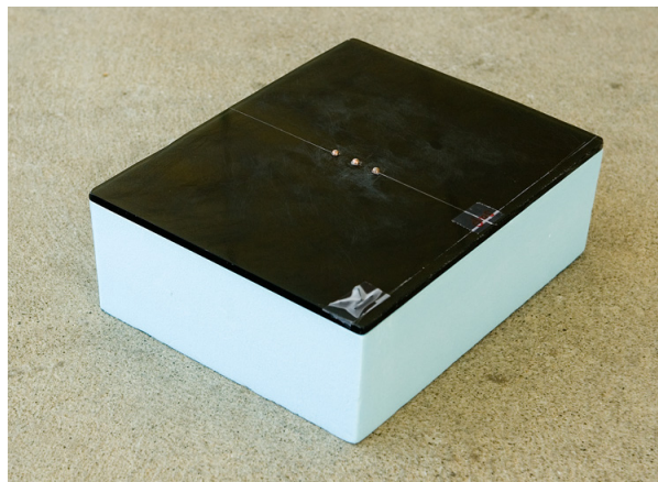
FIG. 7. Morning quality assurance phantom. Consisting of three small steel balls (BBs) mounted half-sunken in a Lucite plate on a Styrofoam base, this phantom is used verify agreement of the isocenters of the kilovoltage and megavoltage beams.
