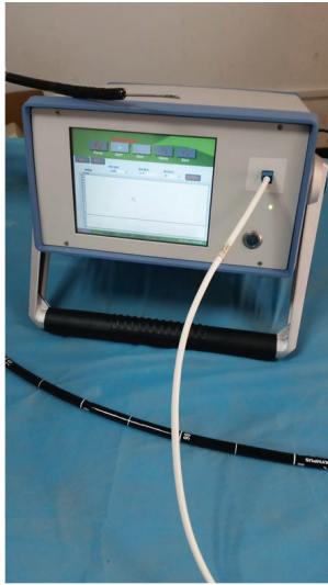
FIGURE 1: Noninvasive measurement of variceal pressure using the endoscopic fibre-optic pressure sensor inserted through the working channel.
