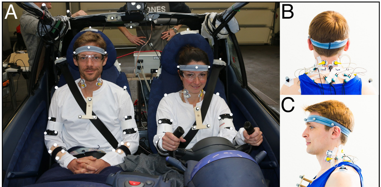
Fig 2. Subjects. (A) Anterior view of subjects sitting in driver and FSP position. Infrared-reflective markers were attached at anatomical landmarks. The LED-flash (at the middle-top of the figure) was triggered when the pendulum hit the bumper. The steering wheel was trimmed to provide a better view for the motion capture cameras. (B) Posterior (C) and lateral view of the subjects. The EMG electrodes were placed at the sternocleidomastoid, trapezius, and paraspinal muscles.
