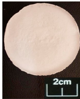
Figure 4. Photographic appearance of the PLA-PVA porous bioscaffold.
