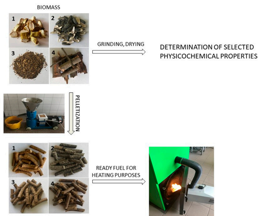
Figure 1. Scheme of the procedure of preparation and use of selected types of biomass as a heating fuel: 1—corn straw, 2—sunflower husk, 3—rapeseed cake, and 4—willow ( Salix viminalis ).
