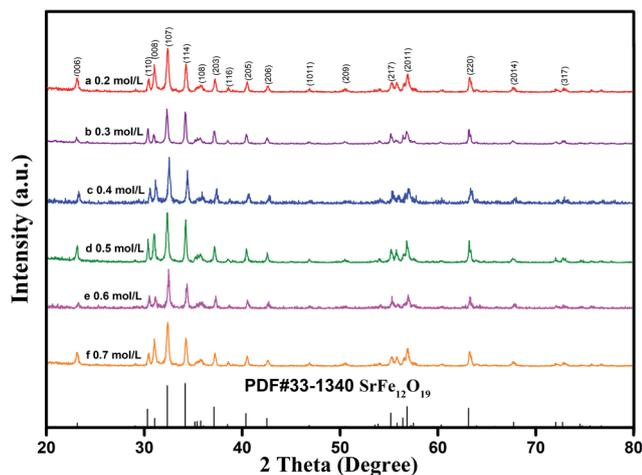
**Fig. 3** XRD patterns of specimens with different initial concentration of ferric ions: (a) 0.2 mol L<sup>-1</sup>; (b) 0.3 mol L<sup>-1</sup>; (c) 0.4 mol L<sup>-1</sup>; (d) 0.5 mol L; (e) 0.6 mol L<sup>-1</sup>; (f) 0.7 mol L<sup>-1</sup> ( $R_{\text{F/S}} = 8$ ).
