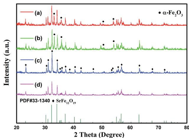
Fig. 1 XRD patterns of specimens with different initial concentration of ferric ions: (a) 0.25 mol L<sup>-1</sup>; (b) 0.375 mol L<sup>-1</sup>; (c) 0.5 mol L<sup>-1</sup>; (d) 0.625 mol L<sup>-1</sup>.
