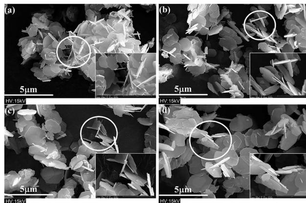
Fig. 11 FESEM micrographs of specimens with different molar ratios of ferric ions to strontium ions: (a)  $R_{\text{F/S}} = 2$ ; (b)  $R_{\text{F/S}} = 3$ ; (c)  $R_{\text{F/S}} = 4$ ; (d)  $R_{\text{F/S}} = 8$ .
