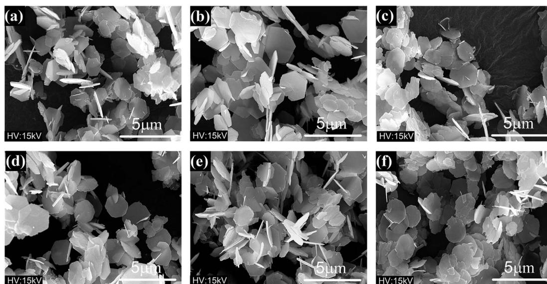
Fig. 7 Typical FESEM micrographs of specimens with various initial concentrations of ferric ions: (a)  $0.2 \text{ mol L}^{-1}$ ; (b)  $0.3 \text{ mol L}^{-1}$ ; (c)  $0.4 \text{ mol L}^{-1}$ ; (d)  $0.5 \text{ mol L}^{-1}$ ; (e)  $0.6 \text{ mol L}^{-1}$ ; (f)  $0.7 \text{ mol L}^{-1}$  ( $R_{\text{F/S}} = 8$ ).
