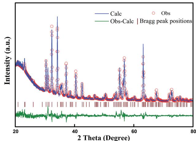
**Fig. 4** The XRD pattern of sample (0.5 mol L<sup>-1</sup>) was fitted by Rietveld.**Table 2** Curie temperature and Rietveld parameters of crystal corresponds to the lattice parameters with different  $c_{\text{Fe}}$
