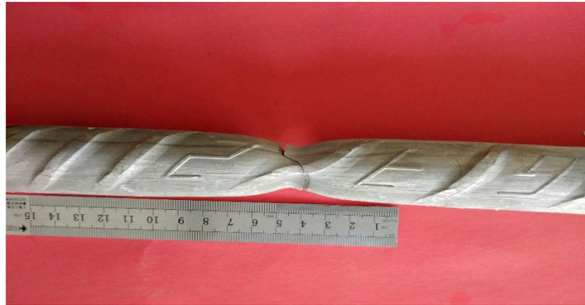
**Figure 1.** Fracture location of duplex stainless steel bars.
