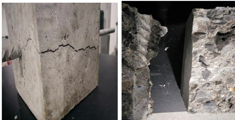
Figure 6. Schematic diagram of cleavage damage.
