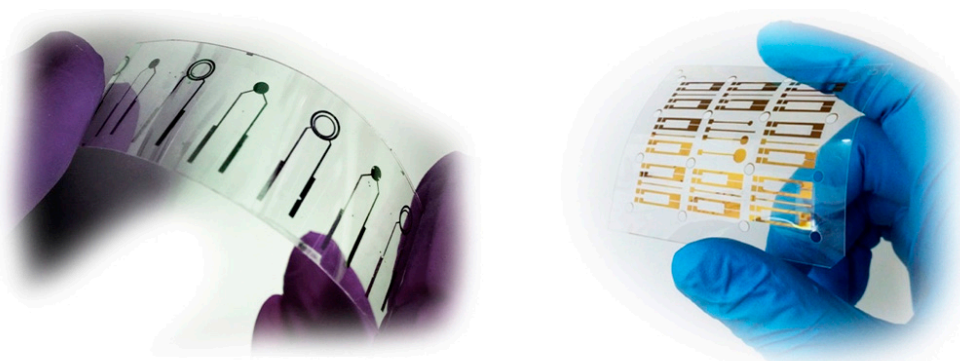
Figure 3. Flexible and disposable thin film field effect devices. Devices produced at CENIMAT/I3N, Universidade Nova de Lisboa by radio frequency magnetron sputtering in low cost flexible substrates according to the procedure described in [55,64].
