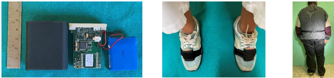
Figure 1. Circuit board of an Inertial Measurement Unit (IMU) and applications.
