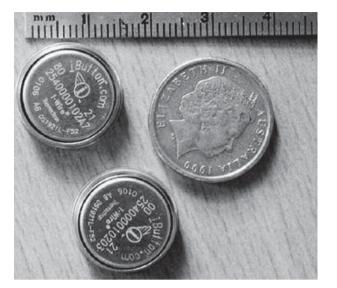
Figure 1. The Thermocron (Maxim Integrated Products, Inc., Sunnyvale, CA, USA) is 15 mm in diameter and is equipped with a temperature sensor, memory, and battery.
