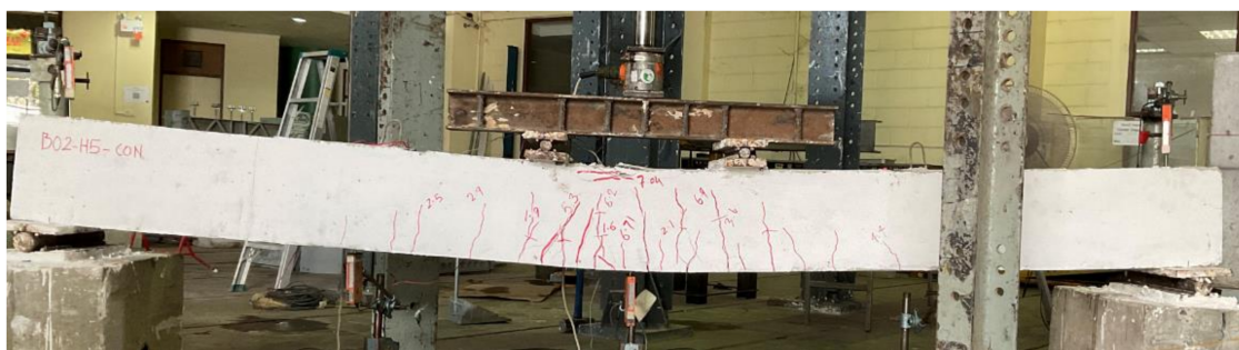
Figure 10. Failure mode of beam B02-HS50-CON.
