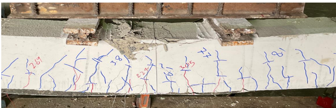
Figure 14. Excessive concrete crushing observed in beam B06-HS100-SCA.
