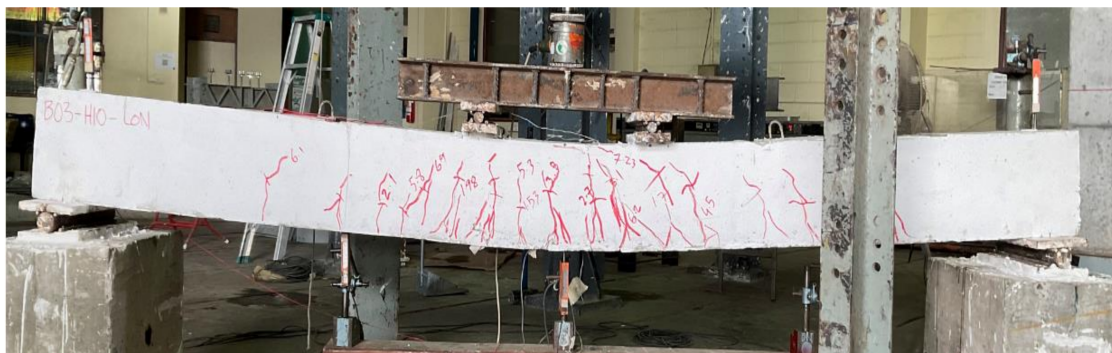
Figure 11. Failure mode of beam B03-HS100-CON.
