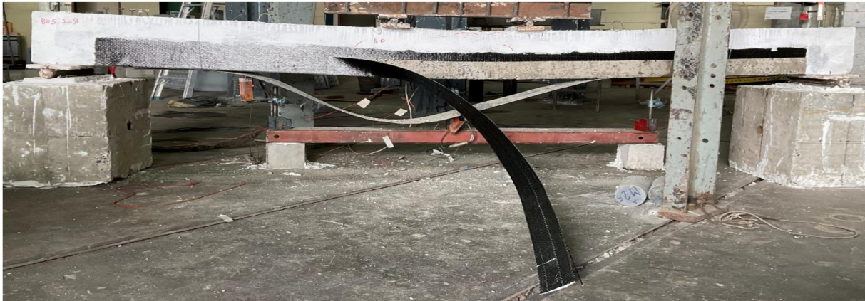
Figure 15. Typical CFRP rupture observed in the 3rd group.
