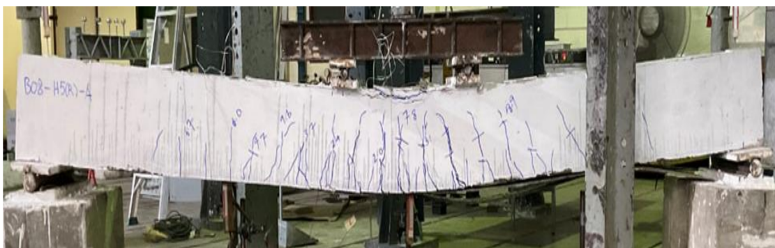
Figure 13. Failure mode of beam B05-HS50-SCA.
