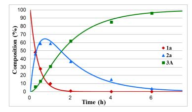
**Figure 1.** Concentration profile for the components during the hydrolysis of dimethyl  $\alpha$ -hydroxybenzylphosphonate (1a) under optimum conditions. The R<sup>2</sup> measure of goodness of fit is 0.994.
