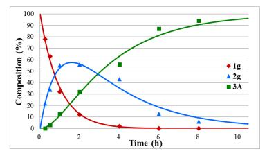
**Figure 2.** Concentration profile for the components during the hydrolysis of diethyl  $\alpha$ -hydroxybenzylphosphonate (**1g**) under optimum conditions. The R<sup>2</sup> measure of goodness of fit is 0.986.
