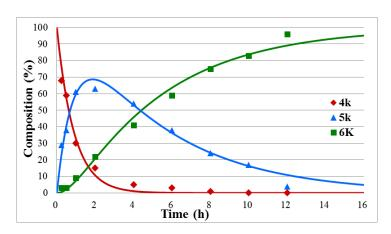
**Figure 3.** Concentration profile for the components during the hydrolysis of diethyl benzylphosphonate (**4k**) under optimum conditions. The  $\mathbb{R}^2$  measure of goodness of fit is 0.983.
