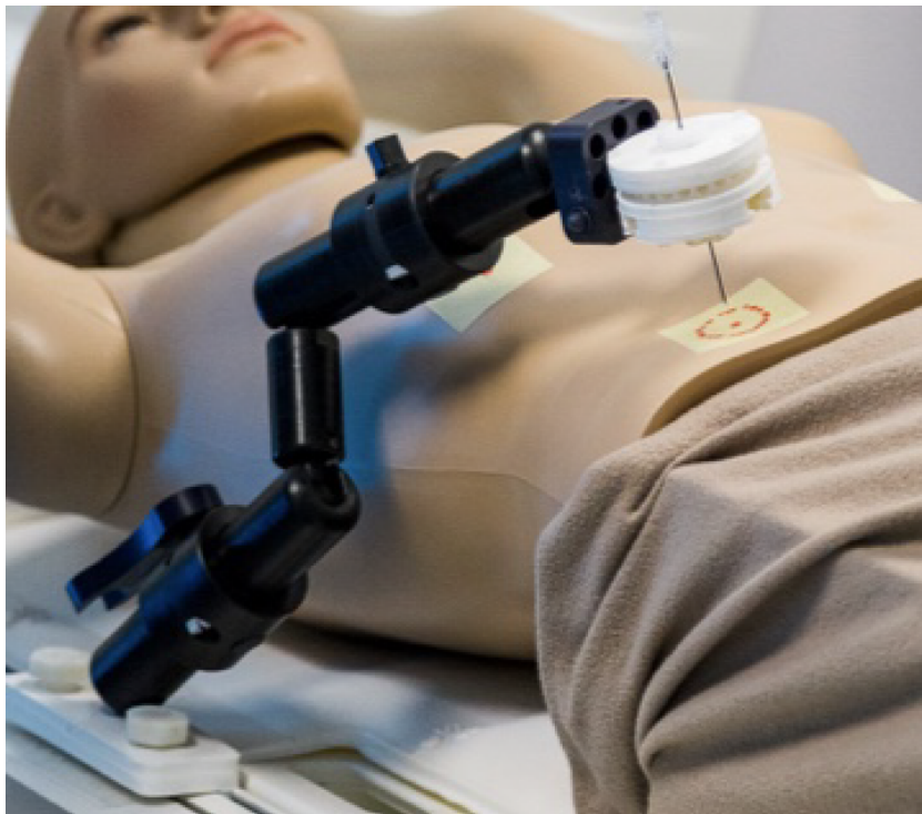
Figure 6 3D printed fully MRI-compatible modular holding arm individually adjustable for procedure needs and patient shape.
