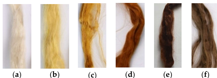
Figure 1. Photographs of cellulose fibers containing silver nanoparticles: (a) 0.01%, (b) 0.05%, (c) 0.1%, (d) 1%, (e) 3% synthesized in the presence of polyethyleneimine (PEI); (f) 0.1% synthesized without PEI.
