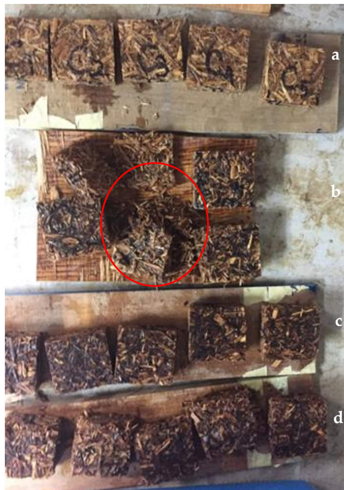
Figure 2. Visual appearance of particleboards after 24 h immersion in water; (a) control, (b) 10 wt% citric acid, (c) 15 wt% citric acid and (d) 20 wt% citric acid, where disintegration of particleboard (red circle) was noticed.
