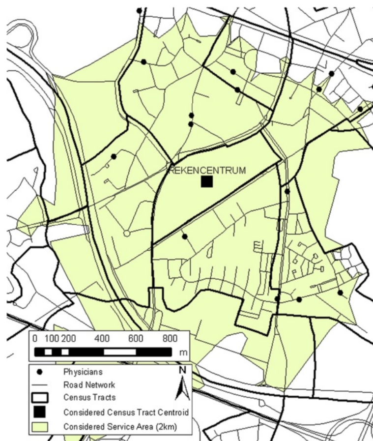
Figure 1 Example of a service area around a census tract centroid, which shows the alignment with the road network and the intersection with the census tract boundaries.
