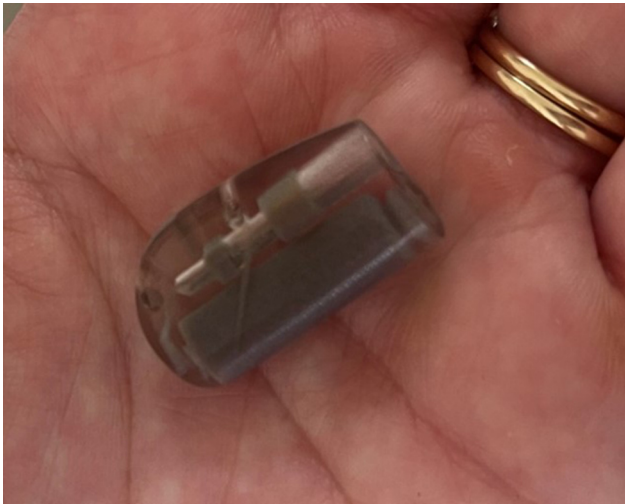
FIGURE 1. Miniaturized adaptor (Medtronic Micra) housing both a bipolar lead socket ( top ) and transvenous miniaturized pacemaker ( bottom ). Dimensions: 29.4 × 16.6 × 9.6 mm; weight: 5 g; volume: 3.5 cc.
