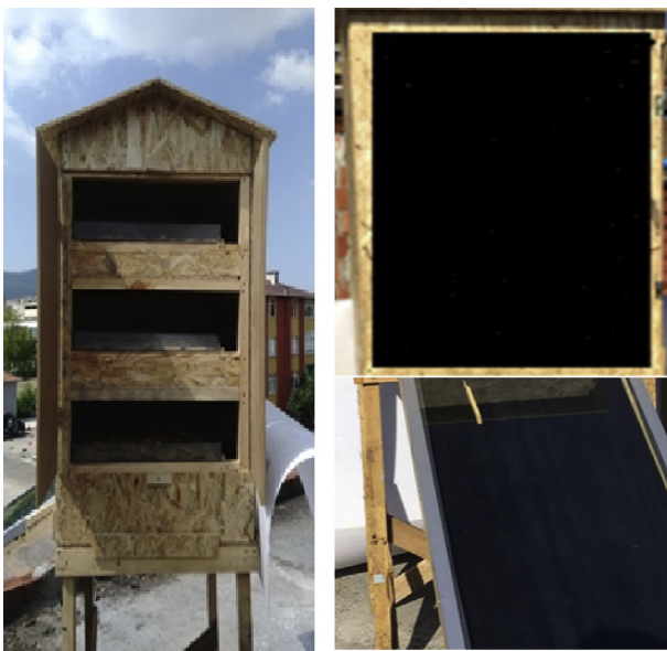
Figure 4. Cost-effective and high-efficient solar drying pilot system prototype.
