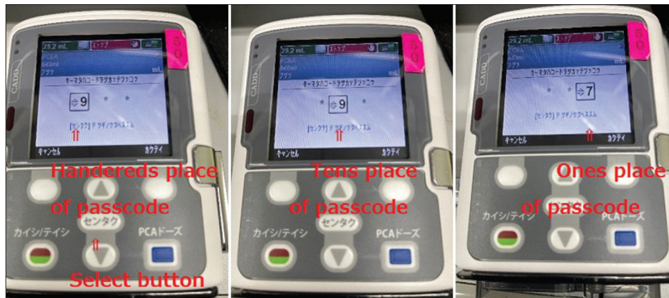
Figure 2: To unlock the PCA pump and change its setting, healthcare providers must ensure that the three-digit passcode with the up-and-down buttons is from hundreds to one place
