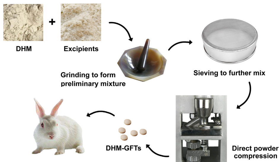
Fig. 2. Schematic representation for the preparation of DHM-GFTs.
