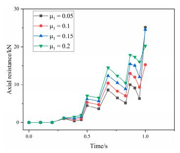
**Figure 14.** The variation of axial resistance between the extrusion ring and fittings body under different friction coefficients.
