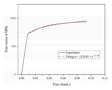
Figure 4. True stress-strain curve and hardening fitting of titanium tube.
