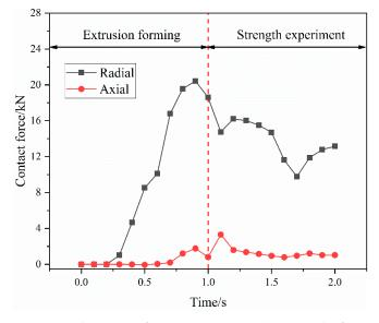
Figure 10. The contact-force variation curve between the fittings body and titanium tube.
