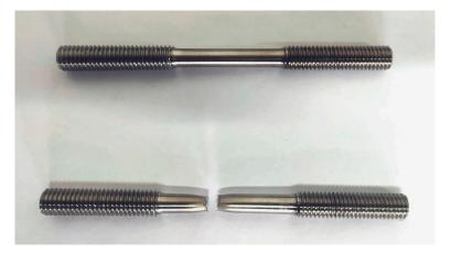
Figure 3. Tensile specimens before and after experiments.
