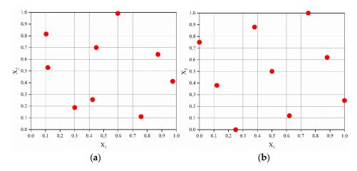
**Figure 16.** Random and optimal Latin hypercube-sampling trial-point distributions: (**a**) random Latin hypercube sampling, (**b**) optimal Latin hypercube sampling.
