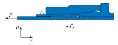
Figure 11. Force analysis on titanium tube during the pull-off process.
