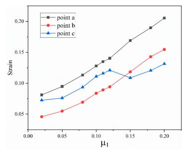
Figure 15. Variation of strain after forming with different friction coefficients at points a, b and c.
