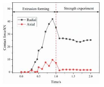
Figure 9. The contact-force variation curve between the extrusion ring and the fittings body.
