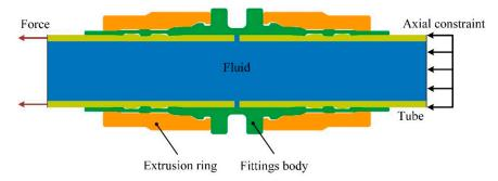
Figure 2. The principle of connection-strength experiment.
