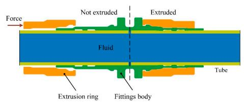
Figure 1. Axial extrusion-joint model.
