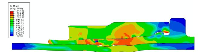
Figure 7. The von Mises stress distribution of axial extrusion joint after extrusion.
