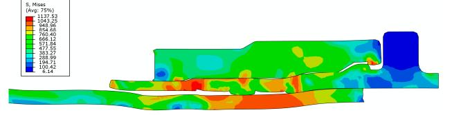
Figure 8. The von Mises stress distribution of axial extrusion joint after connection-strength experiment.
