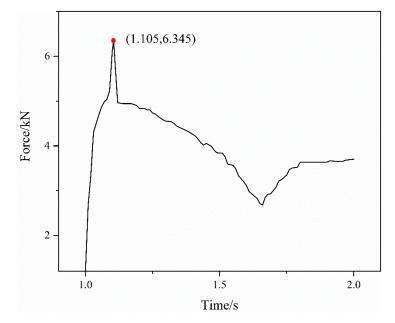
Figure 12. The variation curve of the pulling force on the titanium tube.
