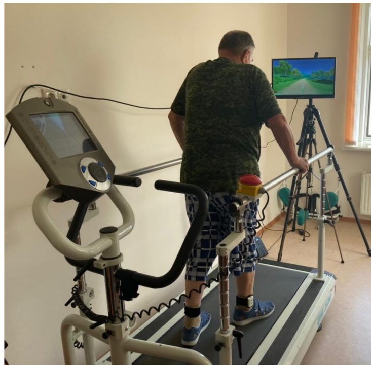
Figure 2. Training process. The patient is on a treadmill. Inertial sensors are installed on his shins to register gait parameters. Before him is a screen with a virtual task.
