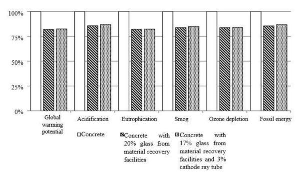
Figure 12. Environmental impact of PC and WG concrete [25].
