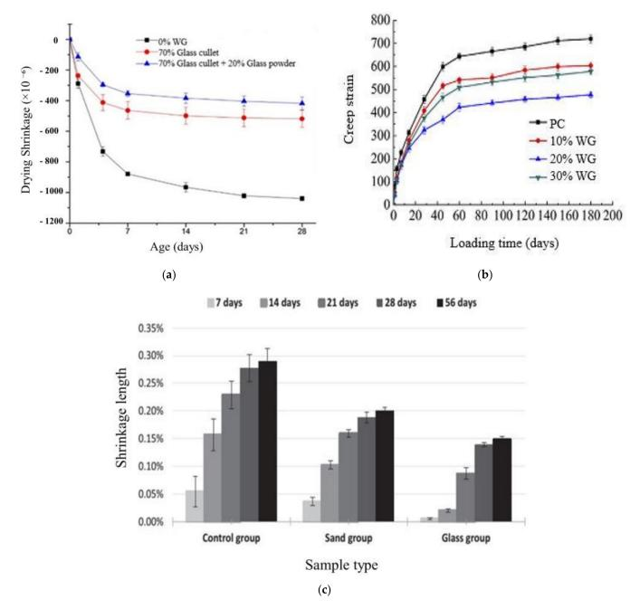
**Figure 6.** Shrinkage properties of cement and geopolymers concretes with WG. (a) Drying shrinkage of concrete with WG [59]. (b) Creep strain of concrete with WG powder [42]. (c) Drying shrinkage of foamed geopolymer concretes with and without fine WG aggregate [45].
