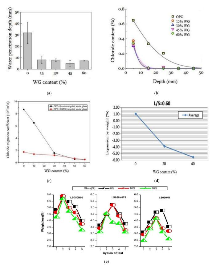
**Figure 7.** Durability of cement and geopolymer concretes with WG powder [73]. (a) Water penetration in WG concrete [41]. (b) Chloride penetration with varying WG contents [41]. (c) Rapid chloride migration coefficient in WG powder-based mortars [34]. (d) Expansion due to sulfate attack in slag-based geopolymer concretes with WG powder [69]. (e) Weight loss in geopolymer concretes with WG powder [73] (LS = liquid to solid ratio, N = % of activator).
