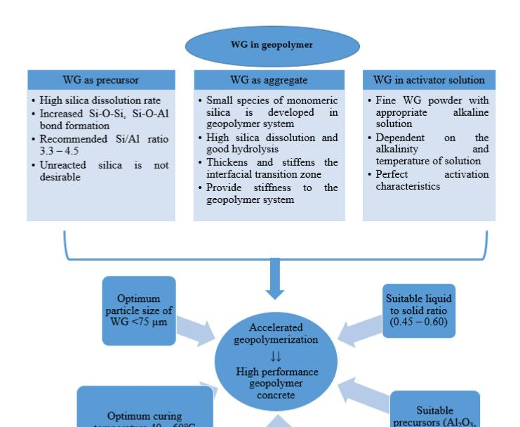
Figure 3. Different roles of WG and the impacts of different parameters on the performance of geopolymer concrete.
