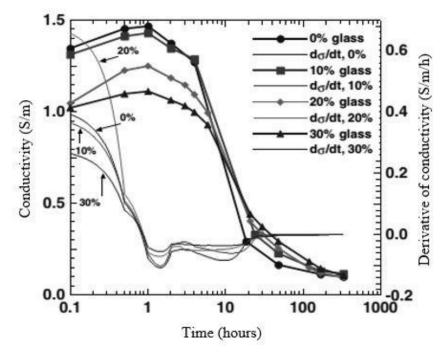
Figure 9. Electrical conductivity of cement–WG powder paste [77].
