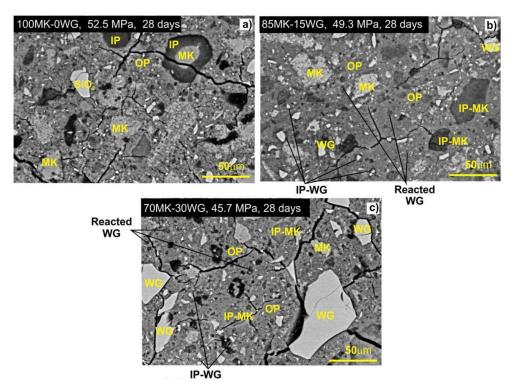
**Figure 5.** SEM of geopolymers with (a) 0%, (b) 15%, and (c) 30% WG at 28 days (activated with sodium silicate modulus Ms = 1.0 and 12% Na<sub>2</sub>O) [7].
