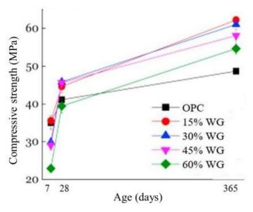
Figure 2. Compressive strength of WGC with WG powder (particles  $< 120 \mu m$ ) as SCM [41].
