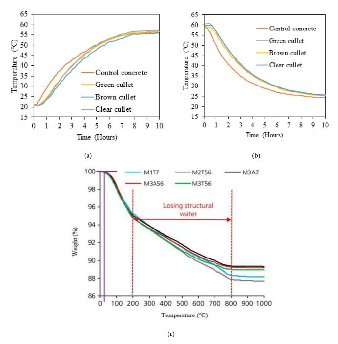
**Figure 10.** Performance of glass-based cement and geopolymer concretes with varying temperatures and times [84]. (a) Variation in WG concrete temperature with varying environmental temperatures (rising) and time [83]. (b) Variation in WG concrete temperature with varying environmental temperatures (falling) and time [83]. (c) Weight loss in geopolymer concretes with varying temperature [84] [M1 with no glass, M2 with 10% and M3 is with 20% glass powder (varying curing condition)].
