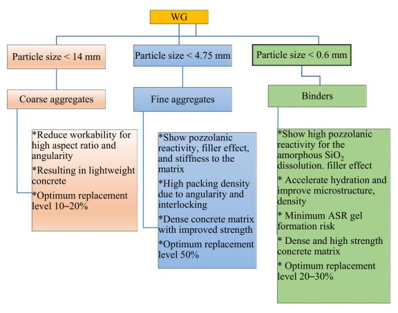
Figure 1. Roles of WG in cement concrete.
