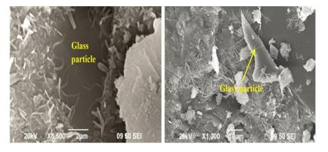
(b) WG particle's mean diameter 28.3 μm
