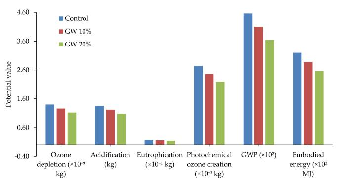
Figure 13. Environmental impact of WG recycled cementitious mixture [91].
