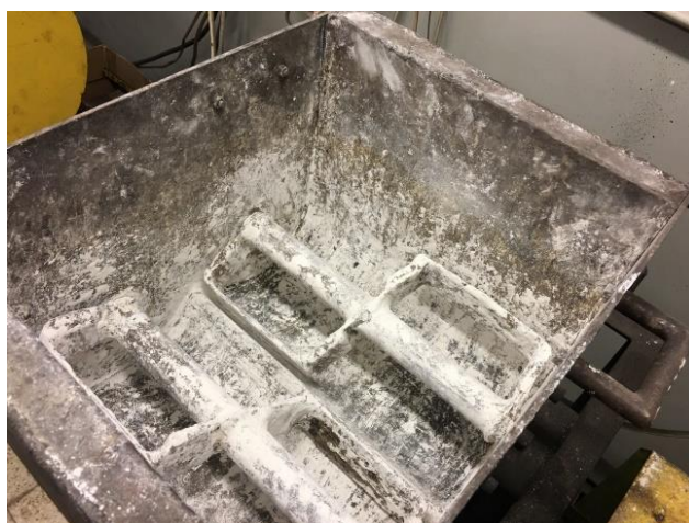
Figure 5. The view of the Z-blade mixer used in the test for material preparation [46].
