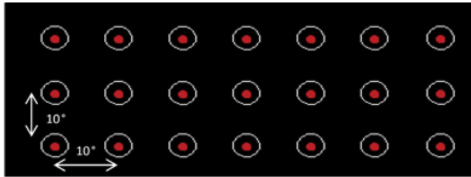
FIGURE 1. Stimulus array configuration with LEDs (red dots) and speakers (white circles) that are 10^\circ apart horizontally and vertically.
