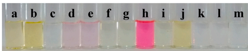
Fig. 1. The color change of (a) P2 ( 1 \times 10^{-5}\text{ M} ) in ethanol upon introducing 1 equiv. of various cations, (b) Ca^{2+} , (c) Cr^{2+} , (d) Fe^{2+} , (e) Fe^{3+} , (f) Co^{2+} , (g) Ni^{2+} , (h) Cu^{2+} , (i) Zn^{2+} , (j) Cd^{2+} , (k) Sn^{2+} , (l) Hg^{2+} , and (m) Pb^{2+} .
