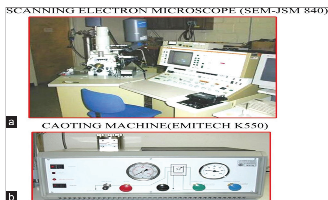
Figure 1: (a) Scanning electron microscope (SEM-JSM 840) used for evaluating the retrieved stainless-steel hardware for surface roughness and corrosion changes (b) EDX study (EMITECH, K550) done to know the composition and metal release from the retrieved stainless-steel hardware
