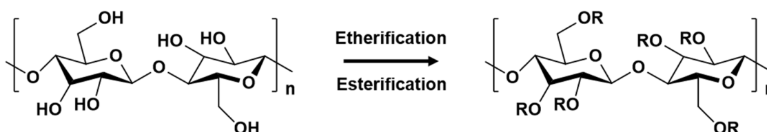
Figure 4. Cellulose is etherified or esterified to form cellulose derivatives.
