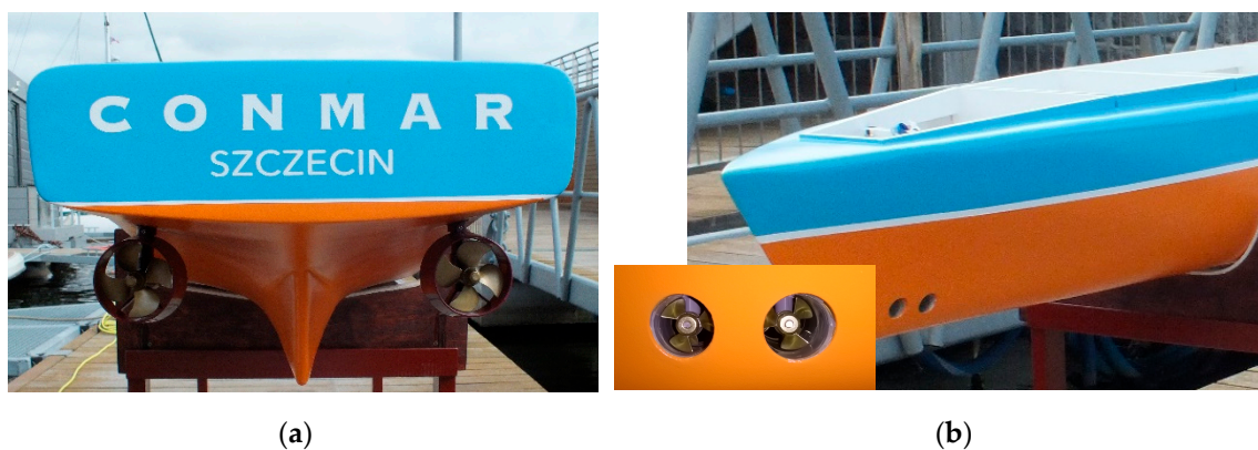
Figure 3. Unmanned vessel model propulsion system: (a) azimuthal stern thrusters, (b) bow tunnel thrusters.
