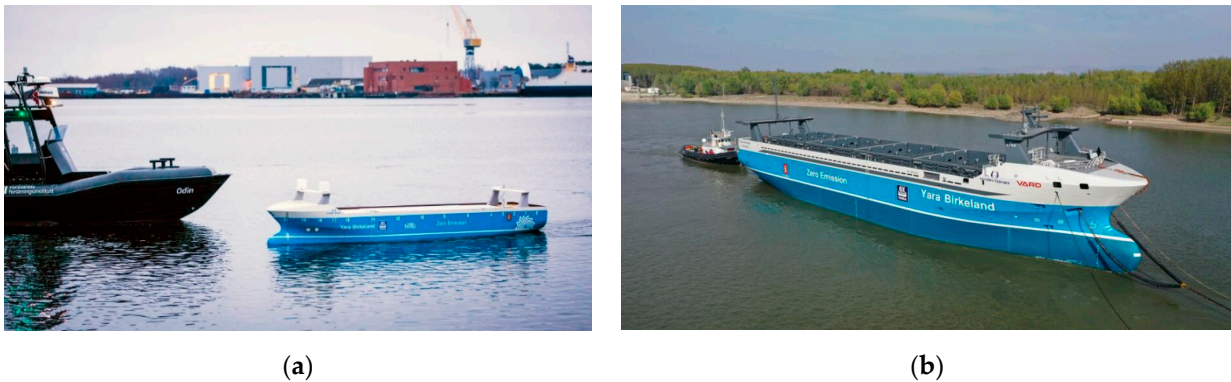
Figure 1. Model of the ship Yara Birkeland for research and testing (a) [9], and the autonomous container ship Yara Birkeland launched in February 2020 (b) [10] (120 TEU, L = 79.5 m, B = 14.8 m).
