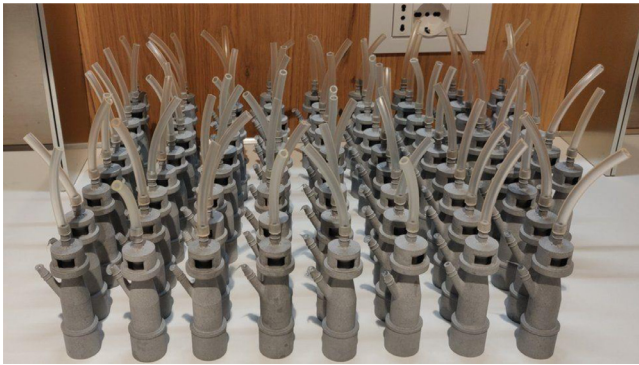
Fig. 7. Respiratory valves developed for Italian hospitals [Reprinted with permission [19].
