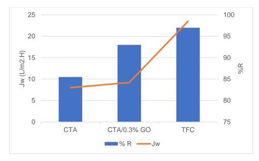
**Figure 13.** Water flux and salt rejection using a natural seawater sample collected from Hurgada– Red Sea coast of Egypt and NaCl as the draw solution (DS) at 25 °C, flowrate1.55 L/min, FO mode: with cells vertically oriented, and active layer—faced feed solution (AL-FS), using Neat CTA, CTA/0.3%GO, and TFC modified membranes.
