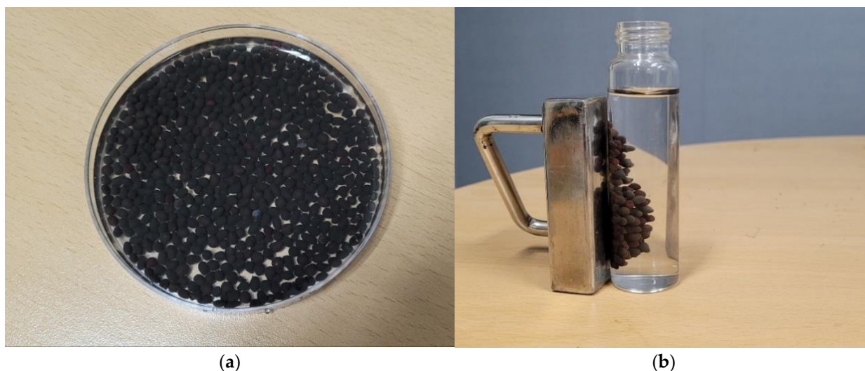
Figure 5. (a) A photo of WFD/SA-PEI and (b) photo to show magnetic properties of WFD/SA-PEI in solutions.
