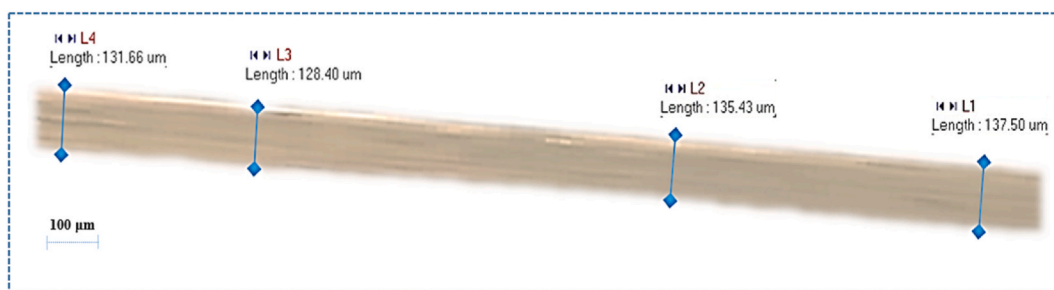
Fig. 5. Ideal microscope image for diameter measurement.
