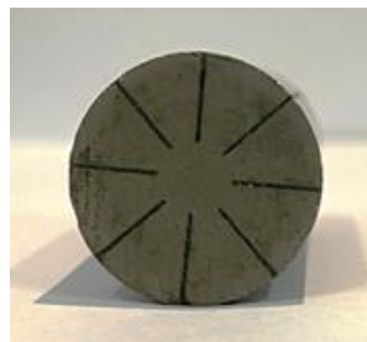
Figure 2. Photo of a radially slotted Terfenol-D rod.
