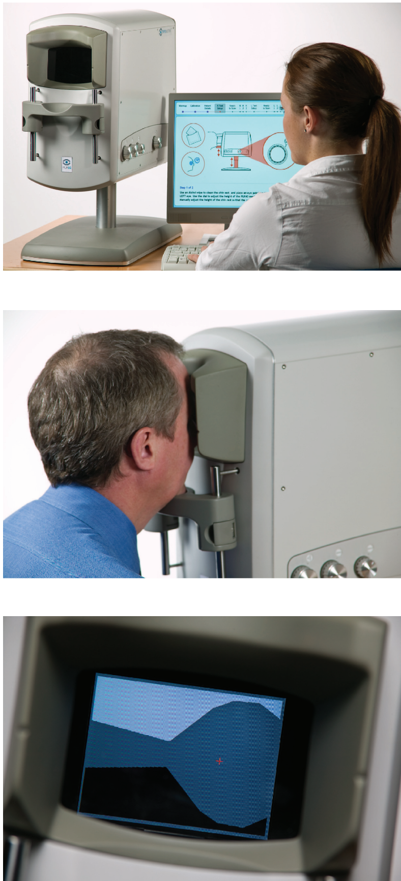
Figure 1 The Pupilmetrix™ PLR60. a) Device layout; b) Patient positioning; c) The peripheral stimulus pattern.
