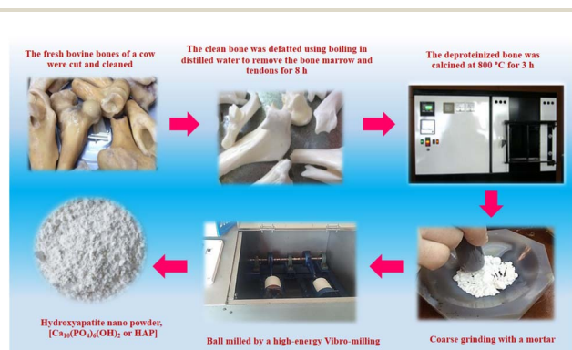
Fig. 1 Schematic of methods to fabricate the nano hydroxyapatite (HAP) powder.
