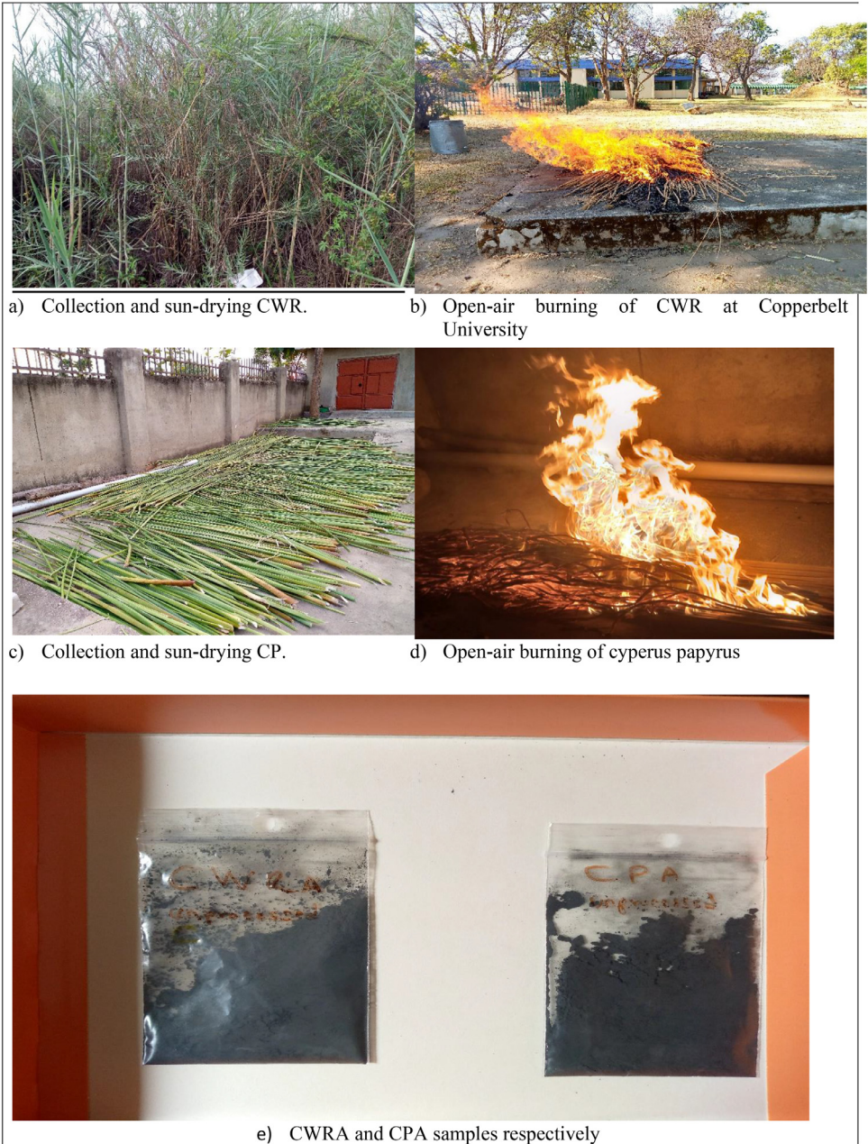
Fig. 3. CWRA and CPA specimen preparation (all the photos were taken by author).
