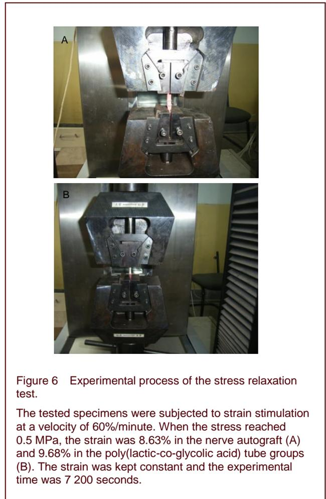
Figure 6 Experimental process of the stress relaxation test.
