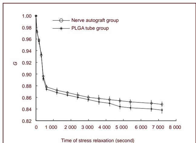
Figure 2 Normalized stress relaxation functions for the nerve autograft and poly(lactic-co-glycolic acid) (PLGA) groups.
