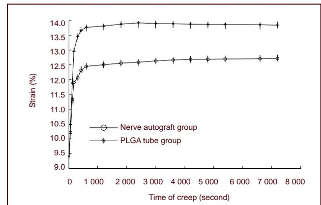
Figure 3 Creep curves of sciatic nerve specimens for the nerve autograft and poly(lactic-co-glycolic acid) (PLGA) groups.
