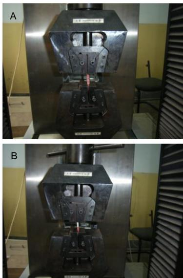
Figure 7 Experimental process of the creep test.
