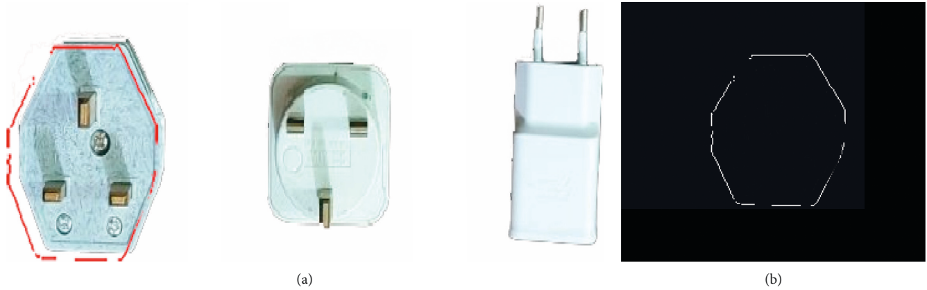
FIGURE 10: The matching of Prewitt edge method: (a) product image captured; (b) template image.
