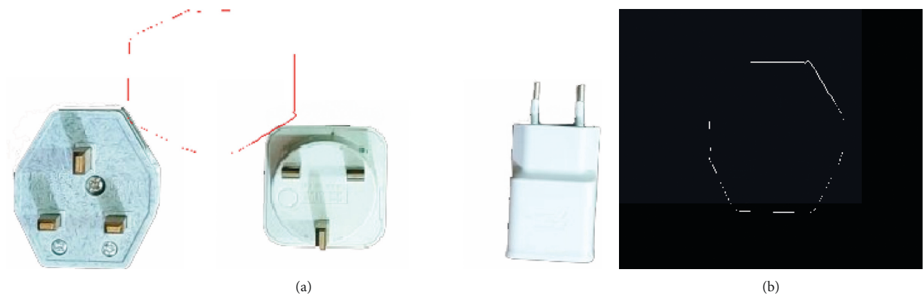
FIGURE 12: The matching of Sobel edge method: (a) product image captured; (b) template image.
