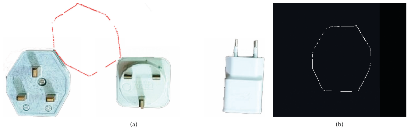
FIGURE 11: The matching of Roberts edge method: (a) product image captured; (b) template image.
