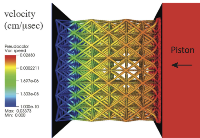
Figure 5. The finite element simulation where the color scale indicated the material velocity. Note: the colors are on a log scale.
