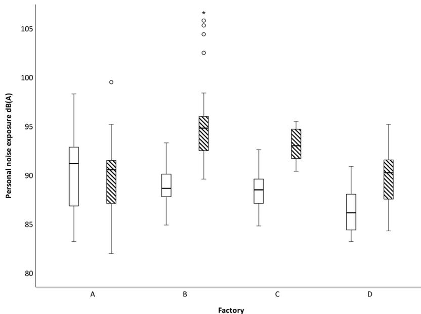
**Figure 1.** Personal noise exposure ( $n = 326$ ) in the furnace (open boxes) and rolling mill (hatched boxes) sections for the four iron and steel factories (A, B, C, and D) in Tanzania. The boxes contain fifty percent of the noise measurements, the solid line within the boxes represents the median value and the whiskers indicate 5th and 95th percentiles, respectively.
